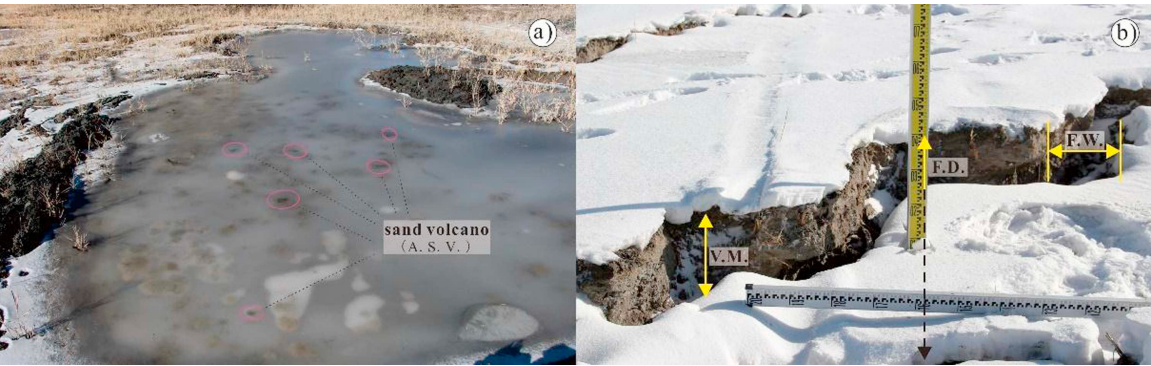
Fig. 7. Schematic diagram of the related measurement parameters. (a) ASV (Table 1). (b) VM, FD, and FW (Table 2).
